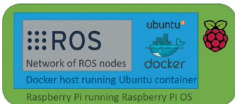
**01** Follow the setup instructions at [magpi.cc/exomysoftware](https://magpi.cc/exomysoftware). This includes the Docker file containing the full software installation.
