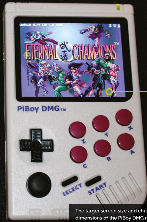
The larger screen size and chunkier dimensions of the PiBoy DMG make it feel like playing a horizontal console despite its vertical form factor
