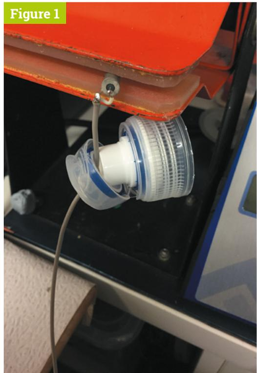
▲ **Figure 1** Soldering the tilt switch to the wire
