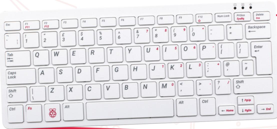
◀ Built entirely into the keyboard, Raspberry Pi 400 keeps clutter to a minimum while simplifying setup – and if you buy the bundled version, it even comes with a Raspberry Pi OS microSD card pre-installed to get you up and running as quickly as possible.
