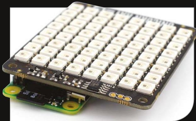
**Left** The small size of the Pi Zero means it's hidden away entirely underneath most HATs, making for a compact build
