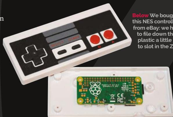
**Below** We bought this NES controller from eBay; we had to file down the plastic a little bit to slot in the Zero
