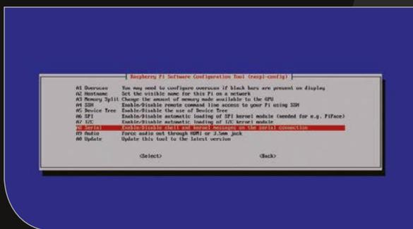
**Above** You'll need to disable the Pi Zero's serial console, which is most easily done through the `raspi-config` utility
