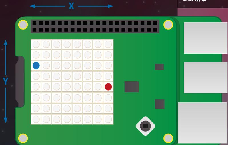
**Fig 2:** The Sense HAT's LED matrix uses a handy coordinate system. The blue pixel is at (0, 0) and the red pixel is at (7, 4)
