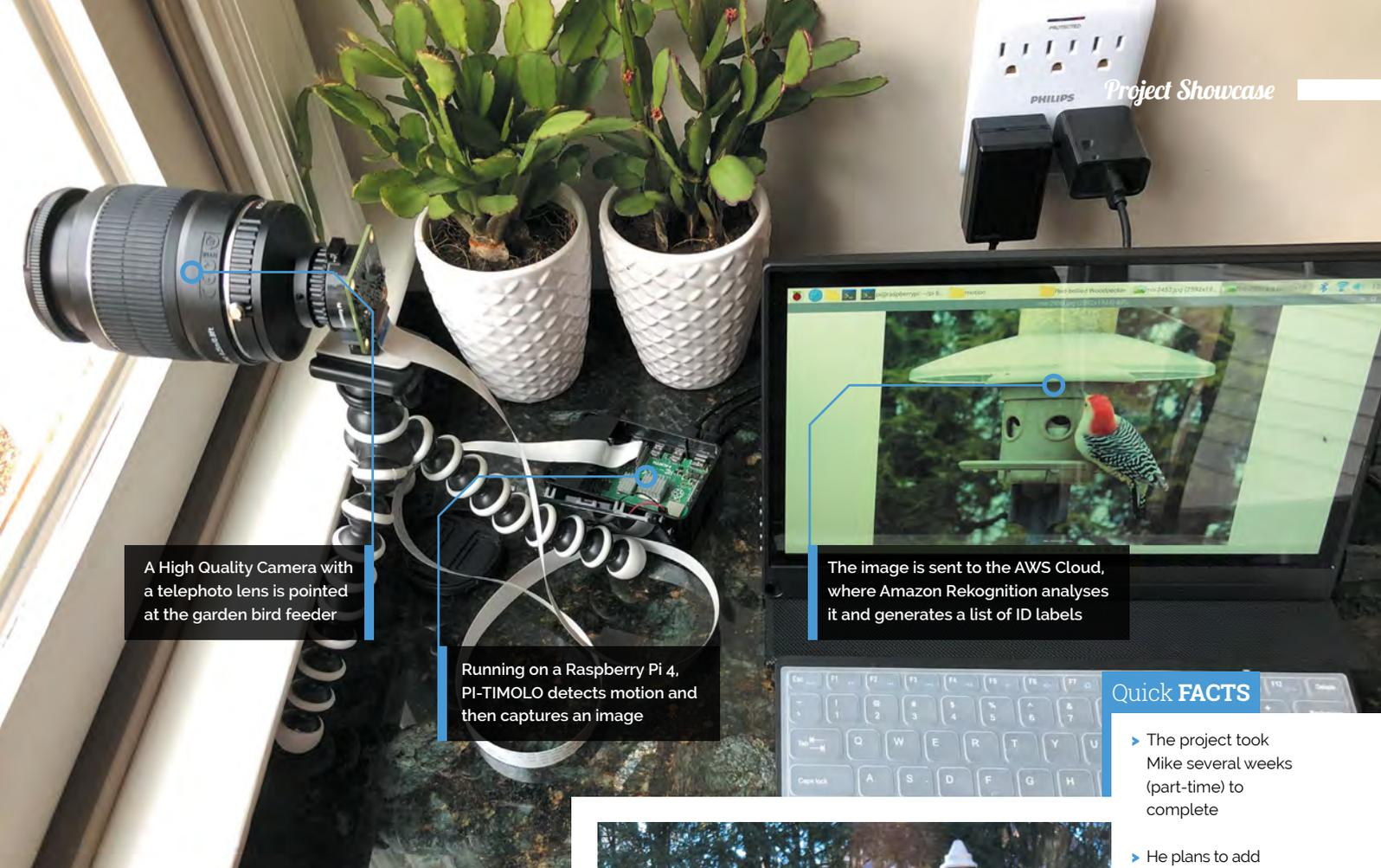
A High Quality Camera with a telephoto lens is pointed at the garden bird feeder
