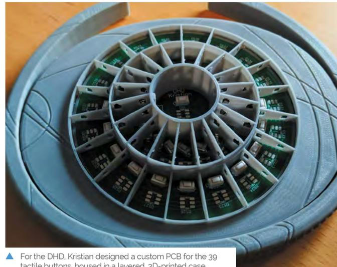
▲ For the DHD, Kristian designed a custom PCB for the 39 tactile buttons, housed in a layered, 3D-printed case
