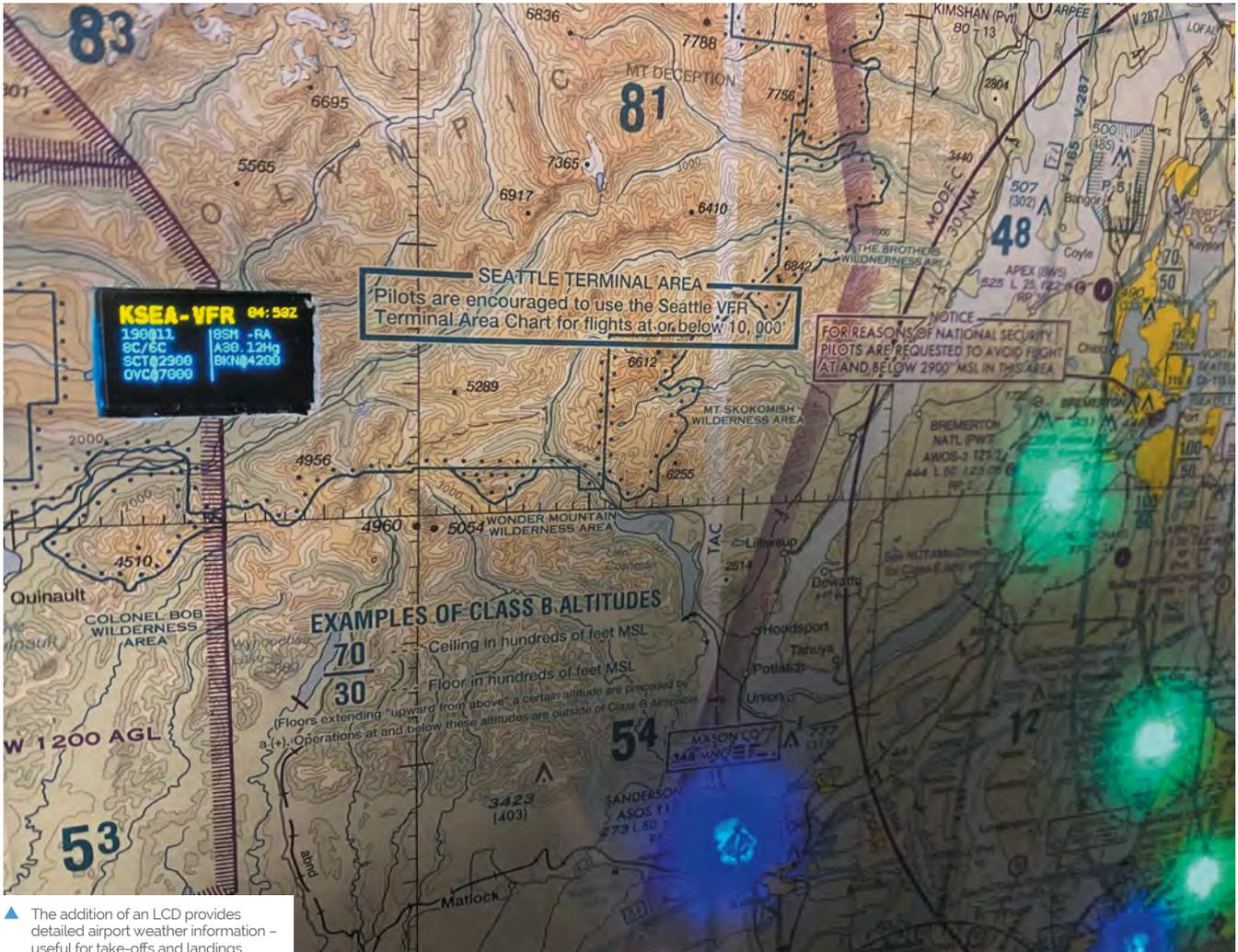
▲ The addition of an LCD provides detailed airport weather information – useful for take-offs and landings
