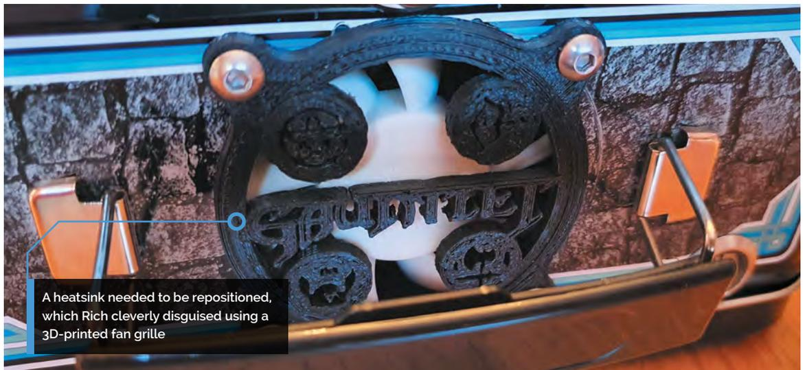
A heatsink needed to be repositioned, which Rich cleverly disguised using a 3D-printed fan grille
