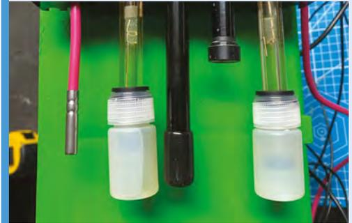
**01** “The entire system has a network of sensors... which monitor atmospheric variables of air temperature, humidity, CO<sub>2</sub>, O<sub>2</sub>, and air pressure. Root zone variables include soil moisture by way of capacitive resistance sensors, reservoir levels by way of float switches, water/soil temperature, water/soil pH, nutrient levels by way of EC, dissolved oxygen, and water quality/root health by way of ORP (oxidation reduction potential).”
