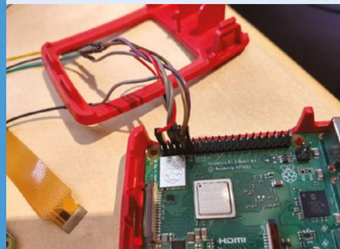
**01** A Raspberry Pi 3B+ was used to trigger the water spray, lights, and fans, bringing an extra element to the gameplay, as well as rendering the arcade machine’s graphics.
