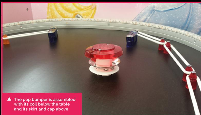
▲ The pop bumper is assembled with its coil below the table and its skirt and cap above
