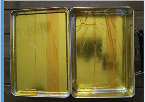
01 One obvious problem with using a metal box is its conductivity, so to avoid any possibility of short circuits, Daniel lined it with Kapton insulating tape before adding the electronics.
