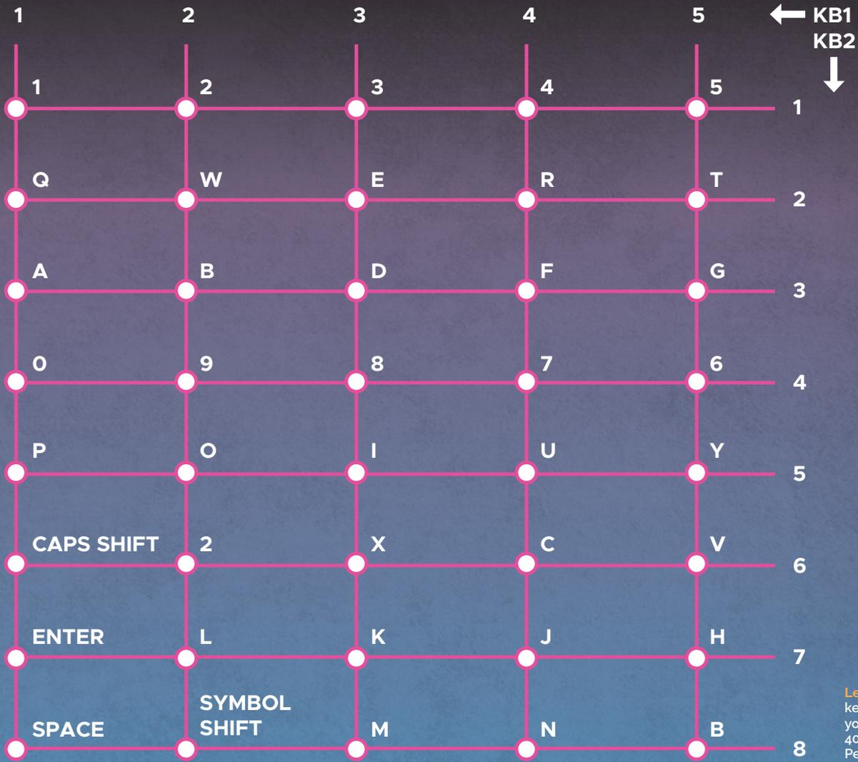
Left The Speccy's keyboard matrix allows you to detect inputs for 40 keys using just 13 lines. Perfect for the GPIO
