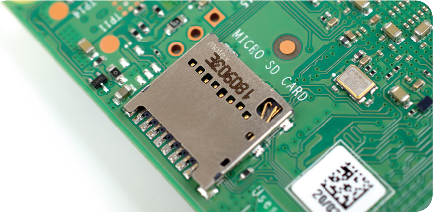
▲ Figura 1-15: Conector microSD do Raspberry Pi
