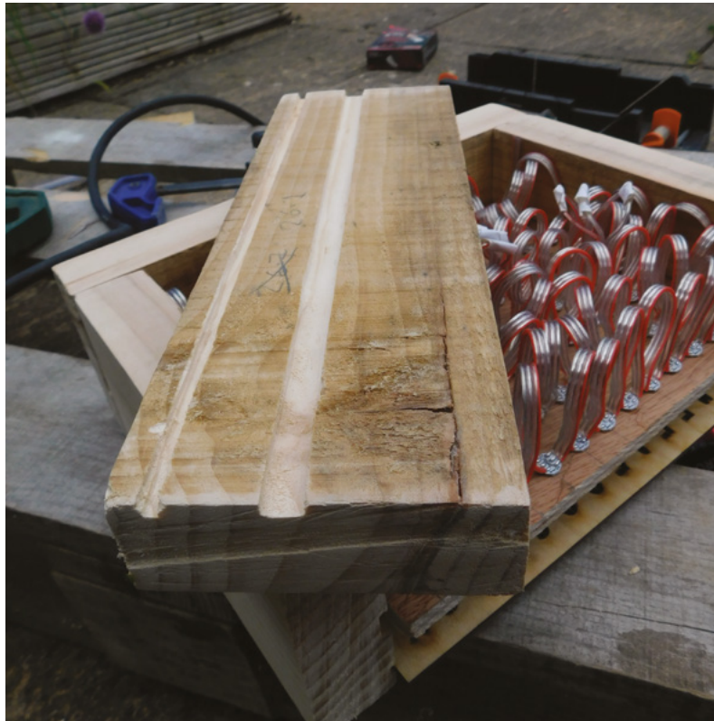
Above ♦ The two grooves routed in our wooden frame to hold the clock face and the LED board
