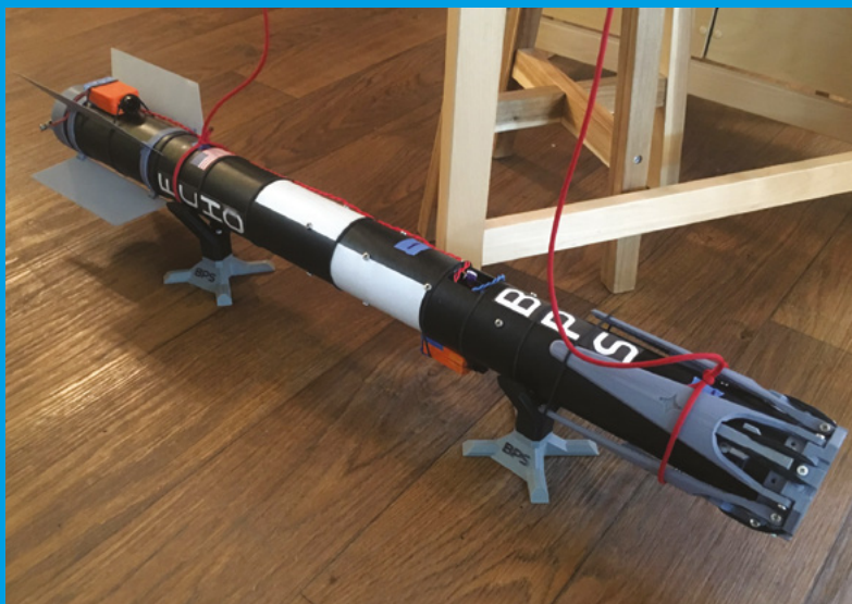
Below ■ The electron rocket that Joe's been attempting to land vertically. Note that the fins are on the top to help stability when coming down
