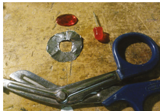
Above ♦ The reflector helps spread the light across the gemstone
