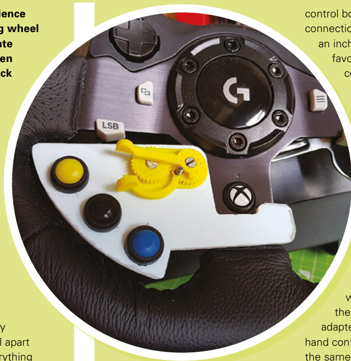
Above ♦ A modified race wheel pedal controller, fitted to a race wheel
