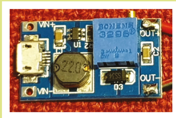
Left Go beyond 5V from USB with a boost converter
