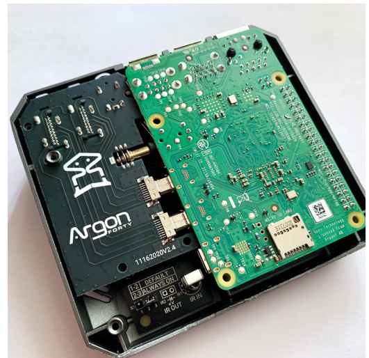
▲ The aluminium case connects to the CPU and memory using thermal paste to act as a giant heatsink
