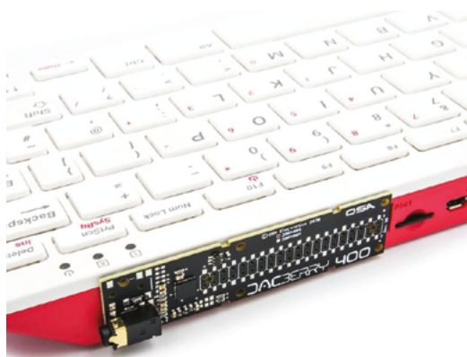
▲ Make sure to connect the board to the GPIO header the right way around and align the pins correctly
