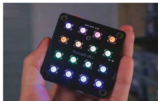
The 4×4 NeoPixel matrix in rainbow cycle mode
