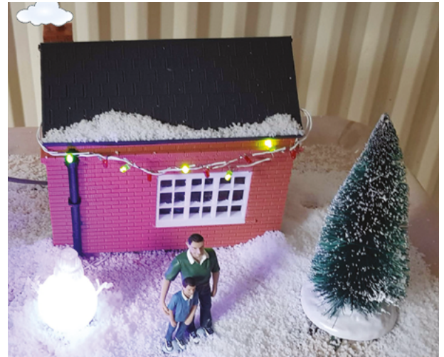
▲ This 3D-printed house had lights controlled via a Raspberry Pi and touchscreen
