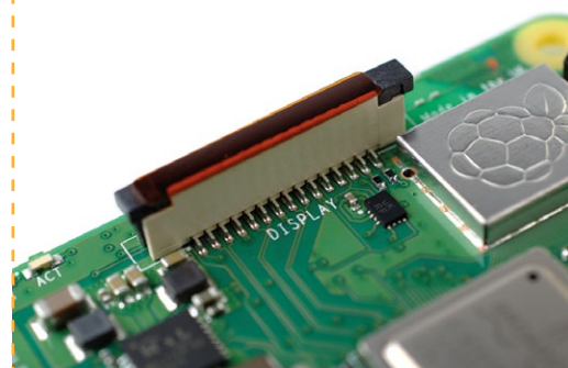
▼ Full-size display (DSI) and camera (CSI) ports make connecting peripherals a snap
