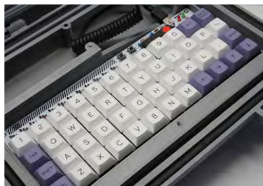
▶ The project uses a compact, smart ortholinear keyboard – that is, one which aligns every key to a strict grid rather than have a staggered key layout
