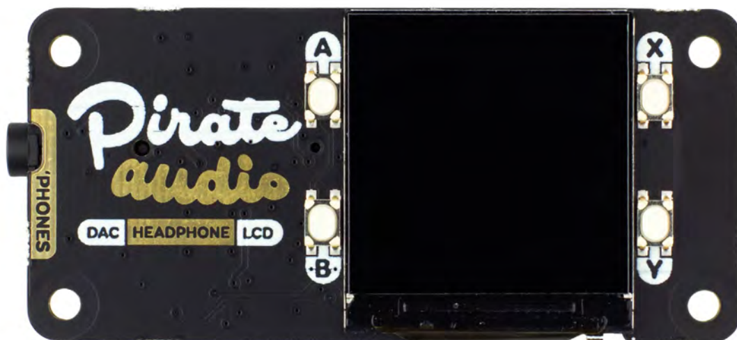
◀ The front of the board features four tiny tactile control buttons on either side of the colour LCD screen
