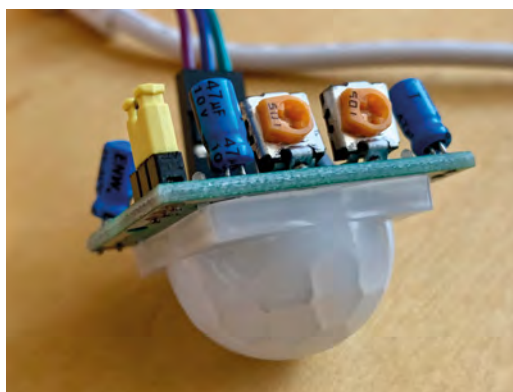
▲ Figure 1 The PIR sensor's potentiometers (orange). Adjust carefully with a small screwdriver, as they can be fragile
