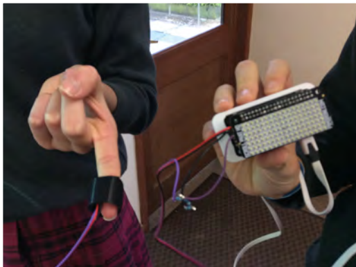
▲ With the pulse sensor attached to a finger, the heart's beats-per-minute can be read
