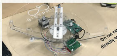
Above The Sisbot works like a CNC cutter, moving the magnet around in circles while the arm moves up and down
